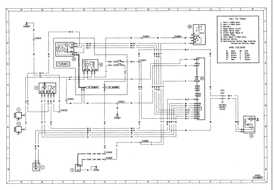
Diagram 3a: Ancillary circuits - horn (R2i and RS models) and wash/wipe
